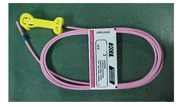
Exel HTD detonators consist of a length of Exel shock tube and a low strength delay detonator. The free end of the tubing is closed with a waterproof seal. The delay detonator is fully enclosed in a unique colour coded handiblock.
